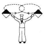
Erase signals, if made by the transmitting station.
